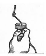
8. Making the hole through the soap Using a screwdriver, make a hole through the soap by slowly rotating and pushing the screwdriver through the soap
