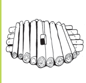
shyira imbaho cyangwa ibiti hejuru yicobo kandi ureebe ngo imbaho cyangwa ibiti bisigaje igice cya mita (50cm) buri ruhande
