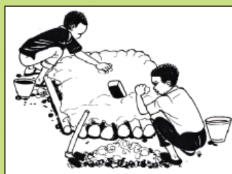
Put mud on the pit
