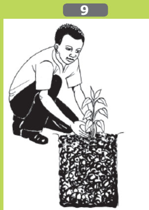
9 When the latrine is full, dig another pit nearby and transfer the superstructure and slab to the new pit. Cover the old pit with soil and plant a fruit tree into the full pit.
