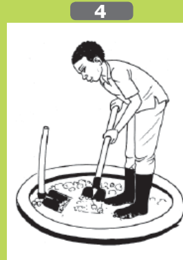
4 Dig pit of about 1 metre or less deep.
