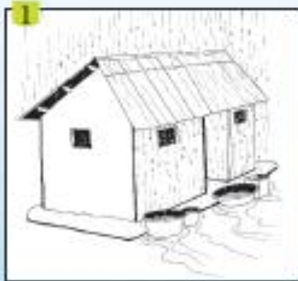
1 Rainwater harvesting without gutters This is not an effective option.
