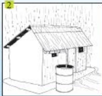
2 Rainwater harvesting in a drum using one gutter
