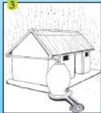
3 Rainwater harvesting with a water jar
